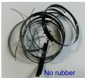
(3) Surface protection (preventing fiber scattering by diameter expansion test)
