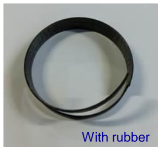
(3) Surface protection (preventing fiber scattering by diameter expansion test)
