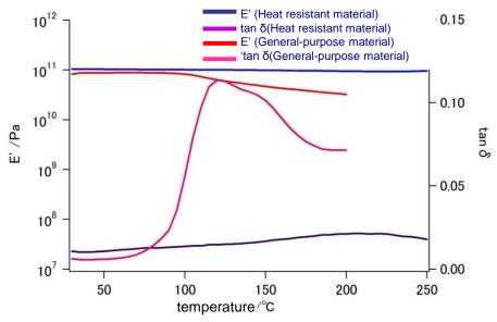
Comparison of heat-resistant materials and general-purpose materials Condition: Three-point bending (1 Hz) Test specimen: Unidirectional laminate thickness = 1 mm
